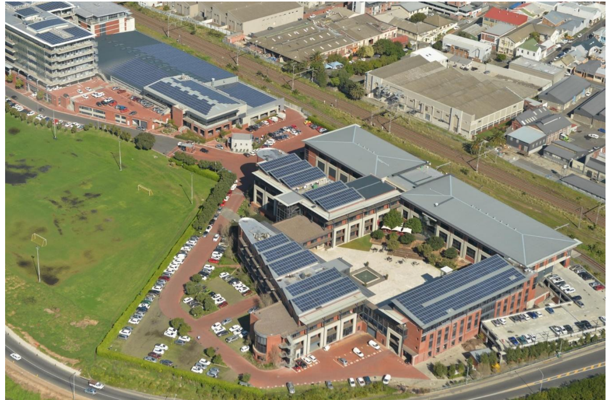
Black River Parkway was the first official grid-tied system with a capacity of 1.2 MW
